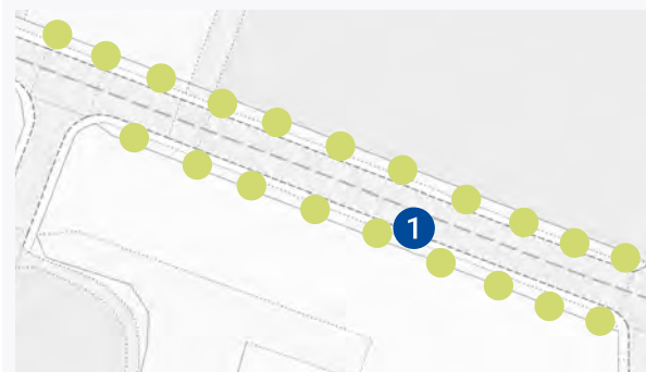
Figure 28 Abbey Road (A4184) Hornbeam boulevard style tree lined street which defines the approach to Evesham town centre at 12m spacing within a 2.4m grass verge. Hornbeam have been used widely in the district.
